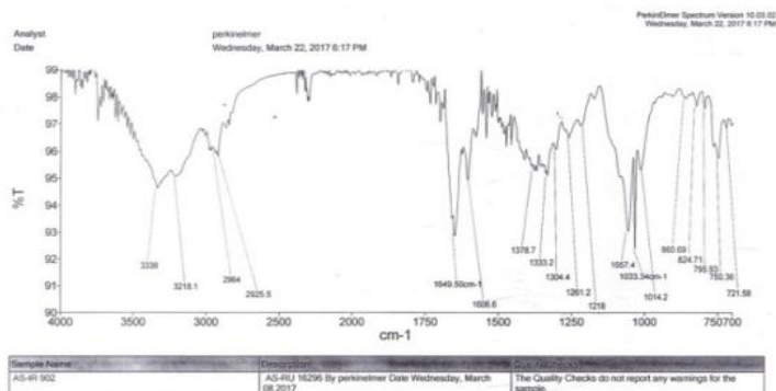
Figure 11. FT-IR spectrum of the isolated compound B
